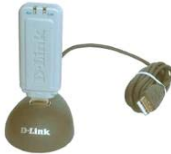
Figure 9: D-Link AirPlus™G DWL-G122 Wireless USB Adapter that support IEEE 802.11b/g protocol.
