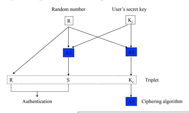
K<sub>c</sub>: ciphering key
