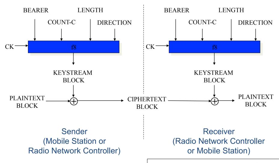
BEARER: radio bearer identifier COUNT-C: ciphering sequence counter
