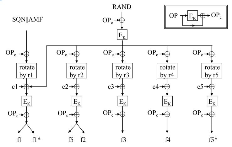
OP: operator-specific parameter r1,..., r5: fixed rotation constants c1,..., c5: fixed addition constants
