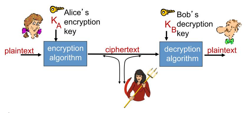
m plaintext message  $K_A(m)$  ciphertext, encrypted with key  $K_A(m)$  $M = K_B(K_A(m))$
